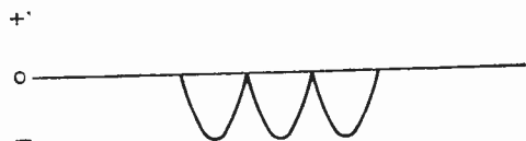
Fig. 7: The waveform obtained when terminal A is held at steady voltage instead of B.
